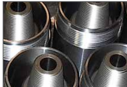
API drill rods and casing subs are typical tooling items
